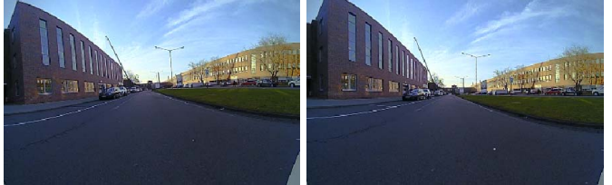
Fig. 7. Cylindrical unwarping, 160-degree horizontal field of view; left: surface not aligned to vehicle; right: surface aligned to vehicle
