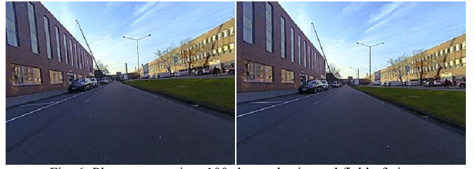
Fig. 6. Planar unwarping, 100-degree horizontal field of view; left: surface not aligned to vehicle; right: surface aligned to vehicle
