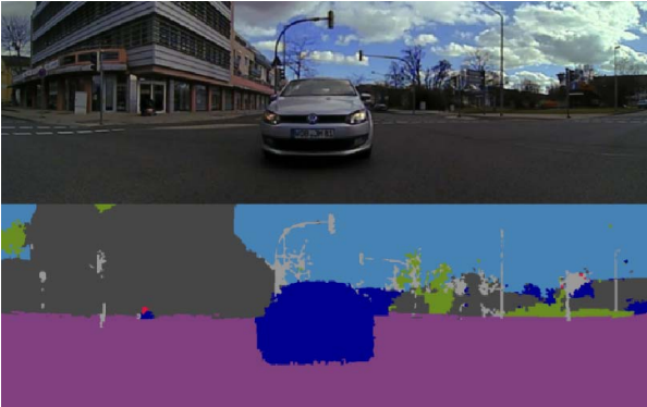
Fig. 2. Cylindrically unwarped rear image and segmentation results
